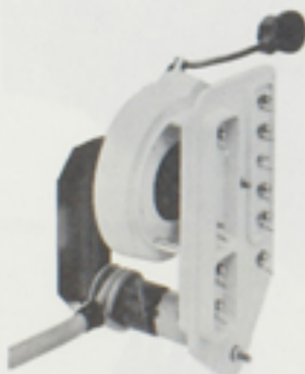
Horizontal deflection (flyback) transformer for color television.
