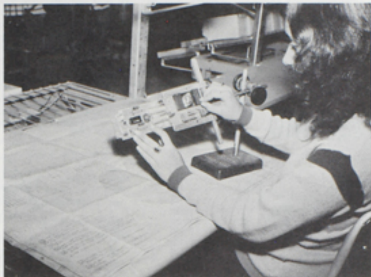
Power supply printed circuit board assembly in Tia Juana plant.
