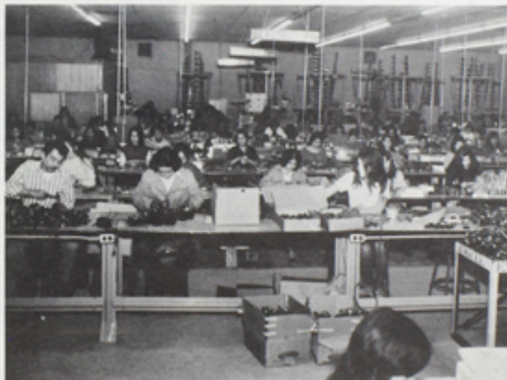
Multiple winding operations and assembly of magnetic components in Tia Juana plant.
