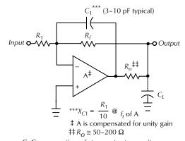
C. Compensation of stray output capacitance. Figure 12-39. Stability enhancement techniques.
