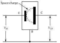
Figure 12-29. Spreading of the space charge between the emitter and the collector, which creates *punch-through*.
