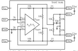
**Figure 12-72.** THAT 1646 block diagram. Courtesy THAT Corporation.
