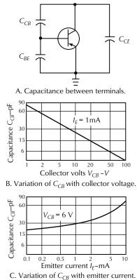
Figure 12-28. Internal capacitance of a transistor.
