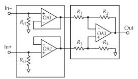
**Figure 12-66.** Instrumentation amplifier. Courtesy THAT Corporation.
