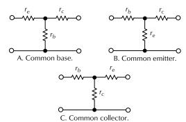
Figure 12-22. Equivalent circuits for transistors.
