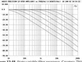
**Figure 12-48.** State-variable filter response. Courtesy THAT Corporation.
