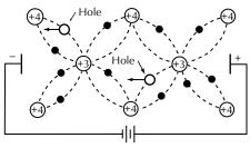
C. Atomic structure of a p-type germanium crystal when a doping agent containing three electrons is induced.
