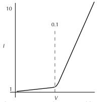
A. Voltage-versus-current characteristic of the junction.
