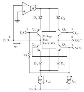
**Figure 12-45.** THAT 2180 equivalent schematic. Courtesy THAT Corporation.
