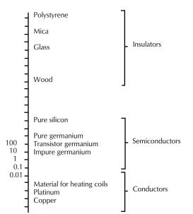
Figure 12-8. Resistance of various materials per cubic centimeter.
