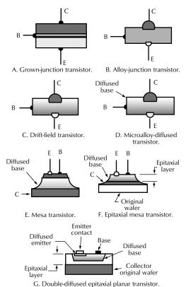
Figure 12-20. Construction of various transistors.
