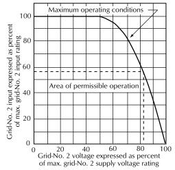
**Figure 12-7.** Typical graph for determining the maximum power dissipated by the screen grid.
