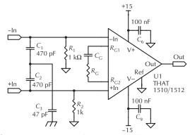
**Figure 12-57.** THAT1510/1512 Basic Application. Courtesy THAT Corporation.
