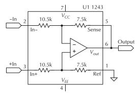
**Figure 12-62.** THAT 1243 with 3 dB attenuation. Courtesy THAT Corporation.
