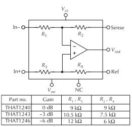
Figure 12-60. 1240 basic circuit. Courtesy THAT Corporation.
