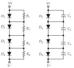
Figure 12-12. Rectifiers connected in series.
