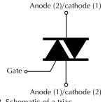
Figure 12-18. Schematic of a triac.
