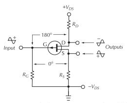
**Figure 12-24.** Signal-voltage polarities in a p-channel field-effect transistor (FET).
