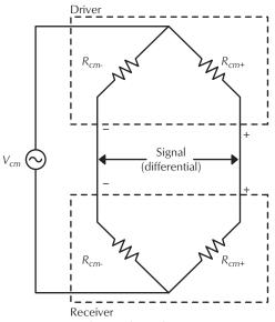
**Figure 12-59.** Balanced Bridge. Courtesy THAT Corporation.
