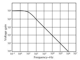
Figure 12-40. Typical open loop gain response.
