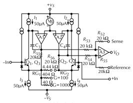
**Figure 12-55.** AD524 block diagram. Courtesy Analog Devices, Inc.
