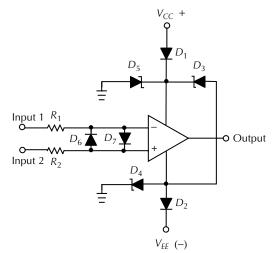
Figure 12-35. Diode protection circuits for op-amps.
