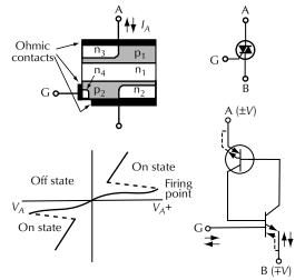
Figure 12-17. Bilateral arrangement to create a triac or ac operating device.
