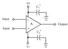
\*Low-inductance short-lead capacitors—0.1 F stacked film preferred. For high-speed op amps, connect  $C_1$  and  $C_2$  directly at supply pins, with low-inductance ground returns.
