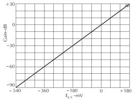
**Figure 12-44.** THAT 2180 gain versus  $E_C^+$ . Courtesy THAT Corporation.
