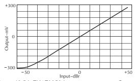
**Figure 12-54.** THAT2252 input versus output. Courtesy THAT Corporation.
