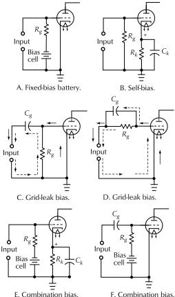
Figure 12-5. Various methods of obtaining grid bias.
