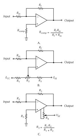
Figure 12-36. Various methods of correcting dc error.
