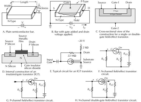
**Figure 12-26.** Basic design circuit for transistor bias circuits.
