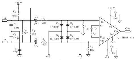
Figure 12-58. THAT preamp circuit with phantom power. Courtesy THAT Corporation.
