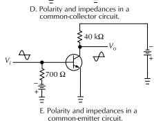
Figure 12-23. Current, polarity. and impedance relationships.
