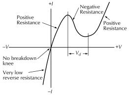
**Figure 12-14.** Tunnel-diode characteristics showing negative region (tunnel region).
