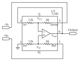
**Figure 12-63.** THAT 1246 with 6 dB gain. Courtesy THAT Corporation.
