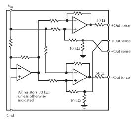
**Figure 12-70.** SSM2142 cross coupled output. Courtesy Analog Devices, Inc.
