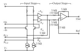
**Figure 12-56.** THAT1510/1512 block diagram. Courtesy THAT Corporation.
