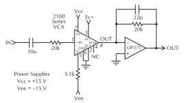
**Figure 12-46.** Basic THAT 2180 VCA application. Courtesy THAT Corporation.
