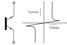
Figure 12-19. Schematic of a diac.
