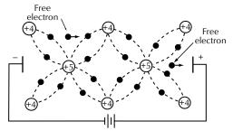
B. Atomic structure of an n-type germanium crystal when a doping agent containing five electrons is induced.
