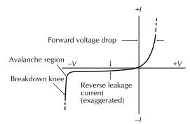
Figure 12-11. Actual diode characteristics.
