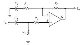
Figure 12-38. A simple noninverting amplifier.
