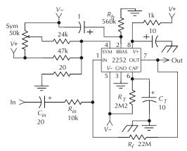
**Figure 12-52.** Typical application of a THAT2252 IC. Courtesy THAT Corporation.
