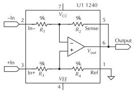
**Figure 12-61.** THAT 1240 with 0 dB gain. Courtesy THAT Corporation.
