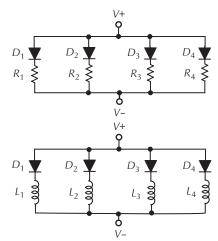
Figure 12-13. Rectifiers connected in parallel.
