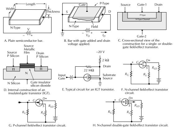
Figure 12-21. Field-effect transistors (FETs).
