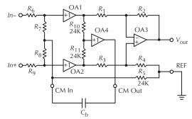
**Figure 12-68.** Balanced line receiver. Courtesy THAT Corporation.
