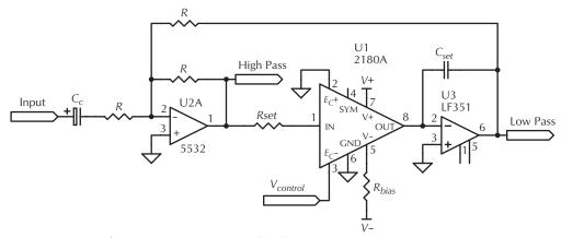
Figure 12-47. VCA state-variable filter. Courtesy THAT Corporation.
