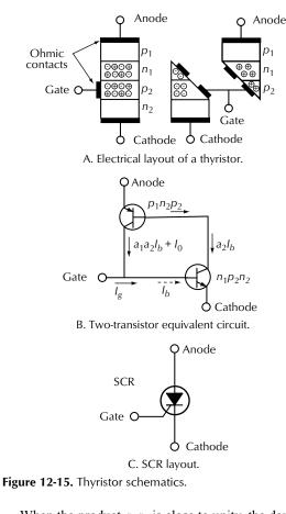
When the product  $a_1a_2$  is close to unity, the denominator approaches zero and  $I_b$  approaches a large value. For a given leakage current  $I_o$ , the gate current to fire the device can be extremely small. Moreover, as  $I_b$ becomes large,  $I_g$  can be removed, and the feedback will sustain the on condition since  $a_1$  and  $a_2$  then approach even closer to unity.
