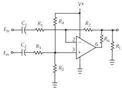
B. Single supply differential amplifier. **Figure 12-41.** Differential amplifiers.
