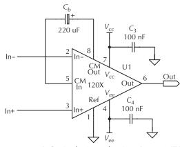
**Figure 12-69.** InGenius basic application. Courtesy THAT Corporation.
