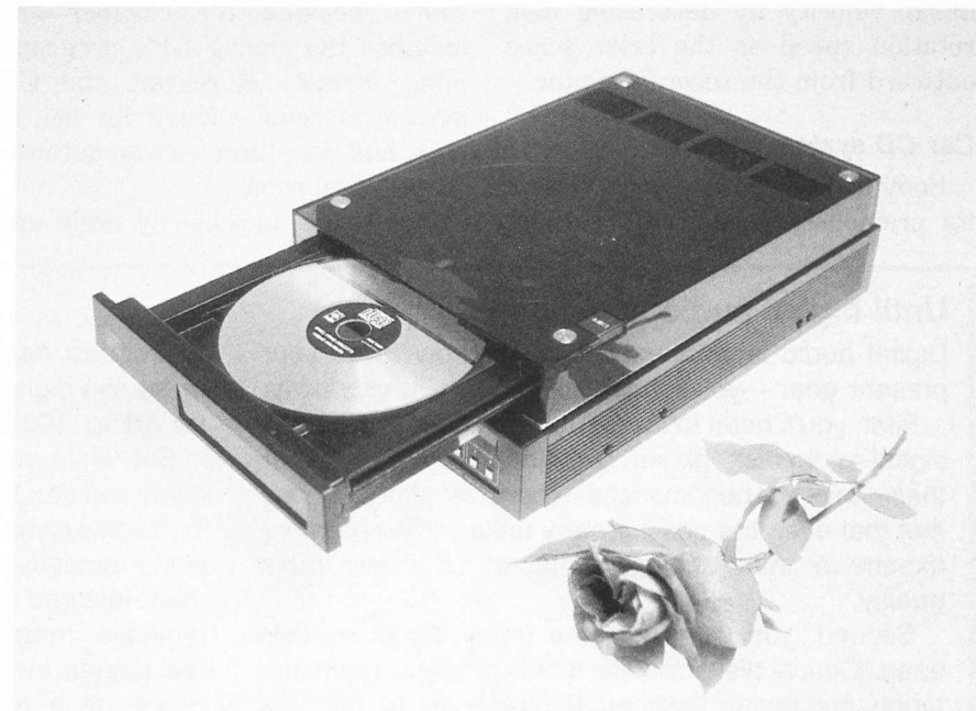
Only 4.7 in. across , the Sony Compact Disk (CD) holds as much as 1 hr of digital stereo audio. CD players should be available in the US by the end of this year.
