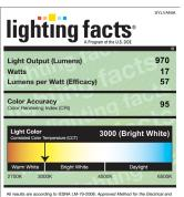
Registration Number: 5BZT-LQ\$YW6 Model Number: LED17PAR30LN/GU24/DIM/P/930\NFL25 Type: Replacement Lamp - Directional (R30, PAR30)
